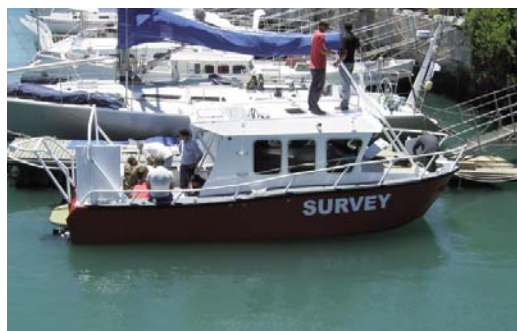
Custom-built catamaran survey spread for shallow water projects
